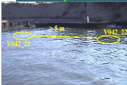
Submerged Targets: grey painted panels 2x2m at 1.5m of depth
