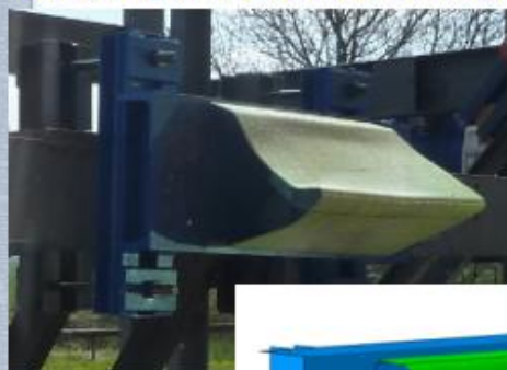
AS01: Calibration Bird Strike Test on Bird Splitter: Good alignment between experiment & prediction
