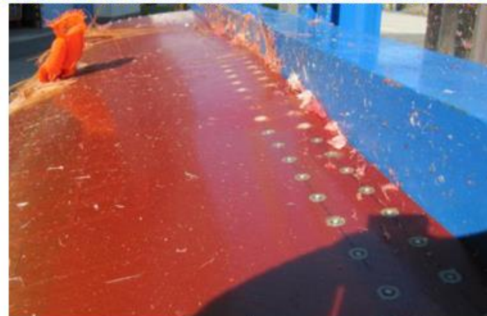
AS01: Repair solution under investigation regarding the AS01 cyclic testing
