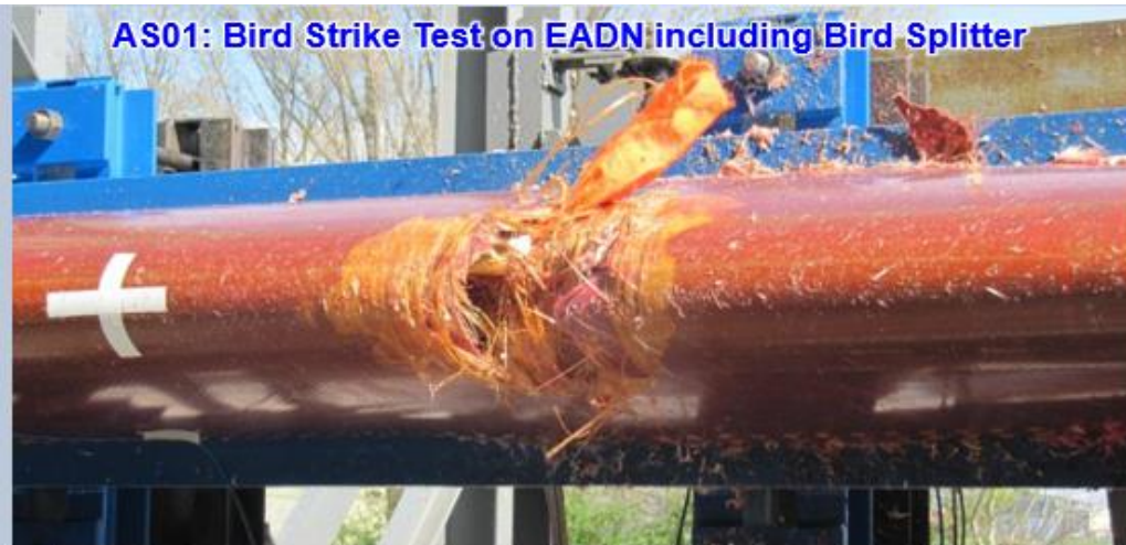
AS01: Calibration Bird Strike Test on Bird Splitter: Good alignment between experiment & prediction
